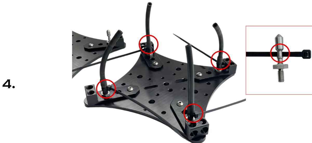
**SECURE THE TUBES USING CABLE-TIES JUST BELOW THE "BULB" OF THE TUBE CONNECTORS.**
