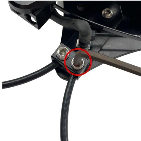
**FIRMLY TIGHTEN ALL 8 SET-SCREWS ONTO THE CABLES.**
