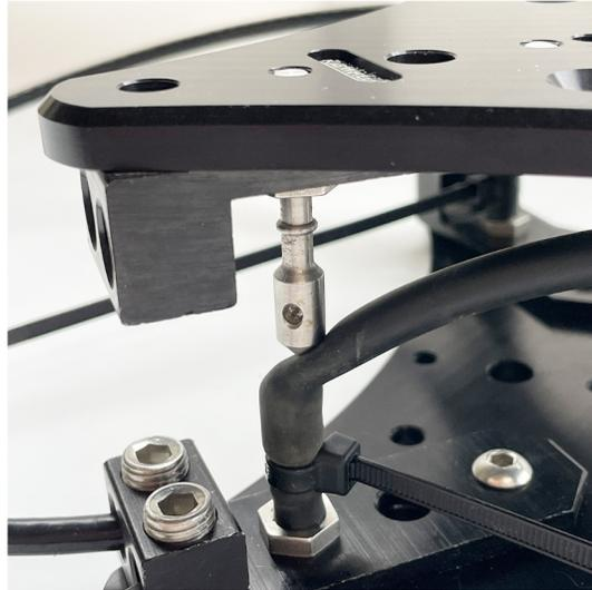
**ATTACH THE LOOSE ENDS OF THE TUBES TO THE CONNECTORS OF THE TOP-PLATE AND SECURE WITH CABLE-TIES.**
